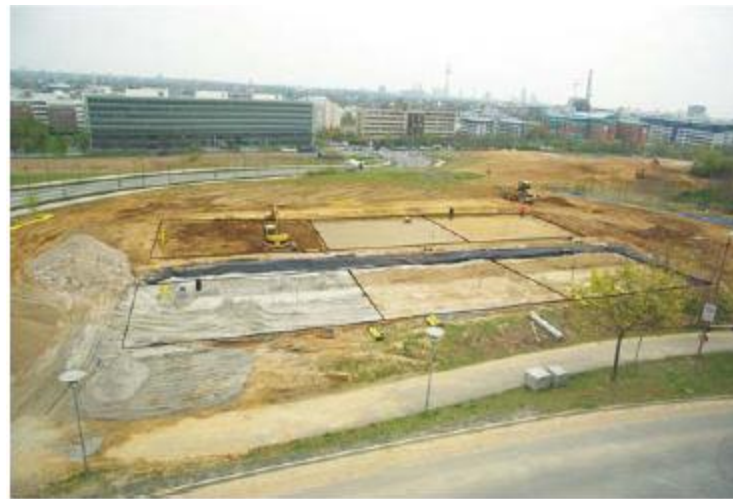
Figure 2: A picture of the test site, taken from the geosciences building on April 21 st 2008. The three areas in front are sealed of the surrounding area by a 2 mm PE-foil.
